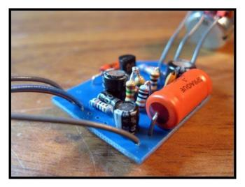
Note the single sided layout lets you use axial or radial caps for C1 and C4. R6 is an on-board current limiting resistor for the LED connections,
