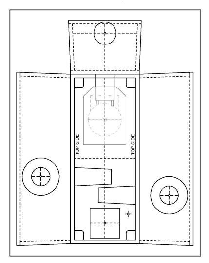
This template is untested. Please check carefully before drilling. Adjustments may be needed in PCB placement. A 9mm Alpha pot will be much easier to fit than a 16mm PCB mounted pot. An external DC jack is also a good choice. Both are available at smallbear.
