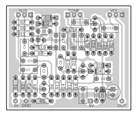
Transistors shown with BC549C pinout. 2.09" W x 1.77" H (including borders)
