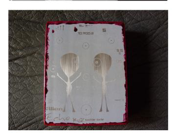
To ensure correct protection of the sides of the enclosure you can conver them with masking tape like this:
