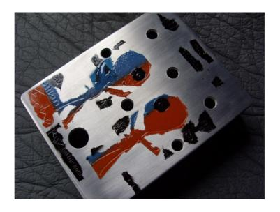
Now remove the paint excess around the designs with 1200 sand paper. Doing it under water will prevent the sanding rests to go into the desings staining the paint.
